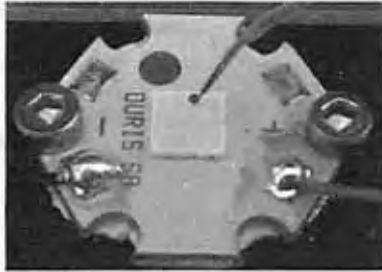
Figure 6: T air Measurement Point (approximately 3mm above LED light source)
